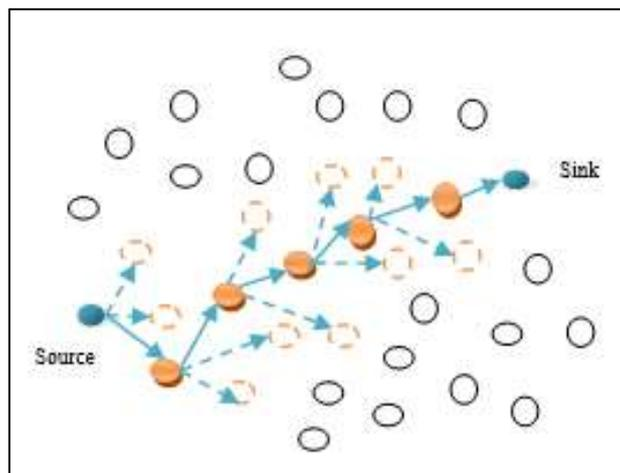
Fig. 2: selection of relay nodes in 1-dimensional.
