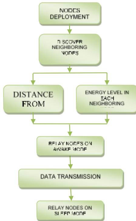
Fig. 1: system design of ENS-OR
