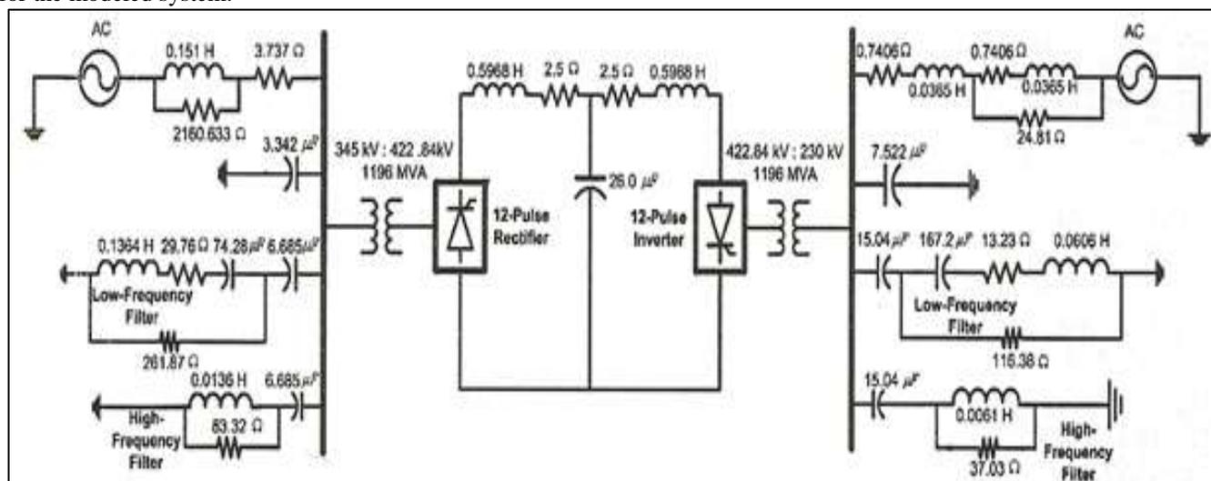
Fig. 3: Single line diagram of CIGRE benchmark HVDC system
