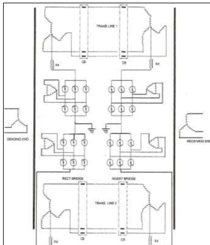
Fig. 1: Basic scheme for simultaneous AC-DC Transmission
