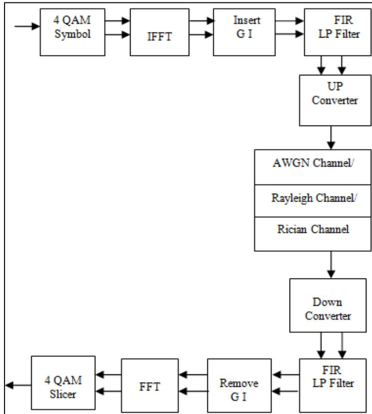
Fig. 2: Block diagram of the simulation model
