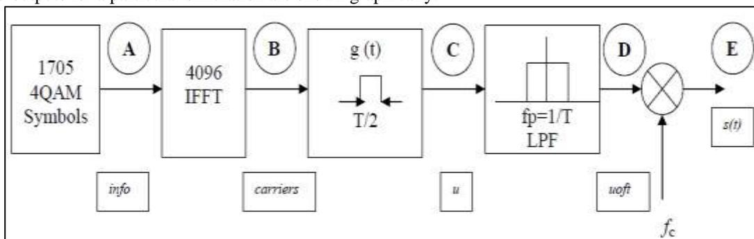
Fig. 3: OFDM symbol generation block diagram [8]
