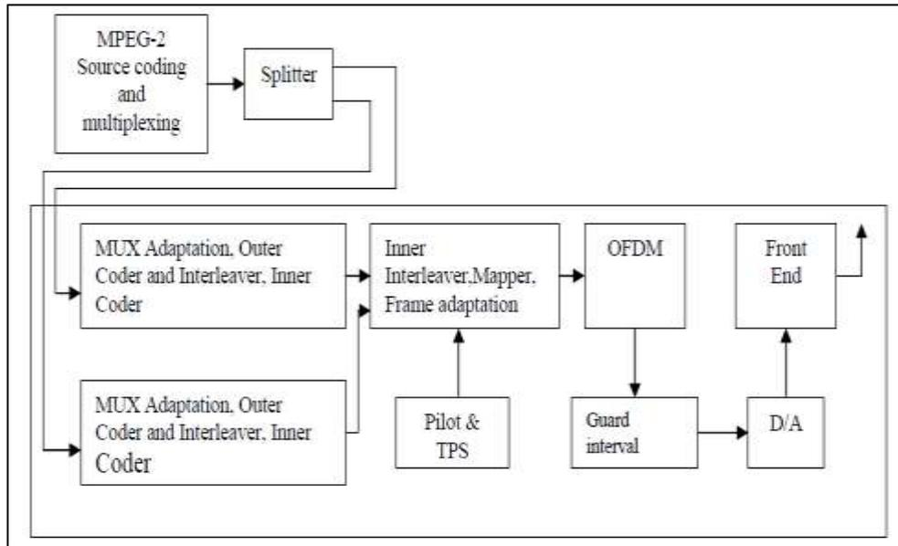
Fig. 1: Terrestrial Digital Video Broadcasting system [4]
