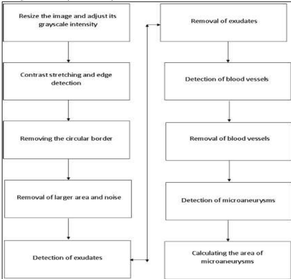
Fig. 5: Block diagram for the detection of micro aneurysms
