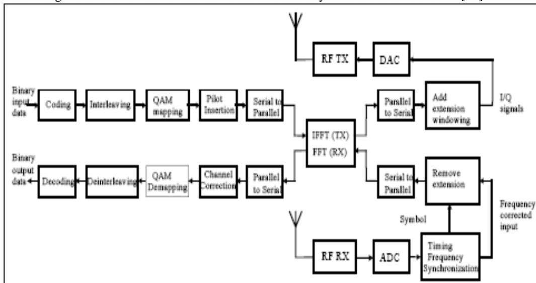
Fig. 4: Channel estimation by pilot carrier technique using MIMO-OFDM system
