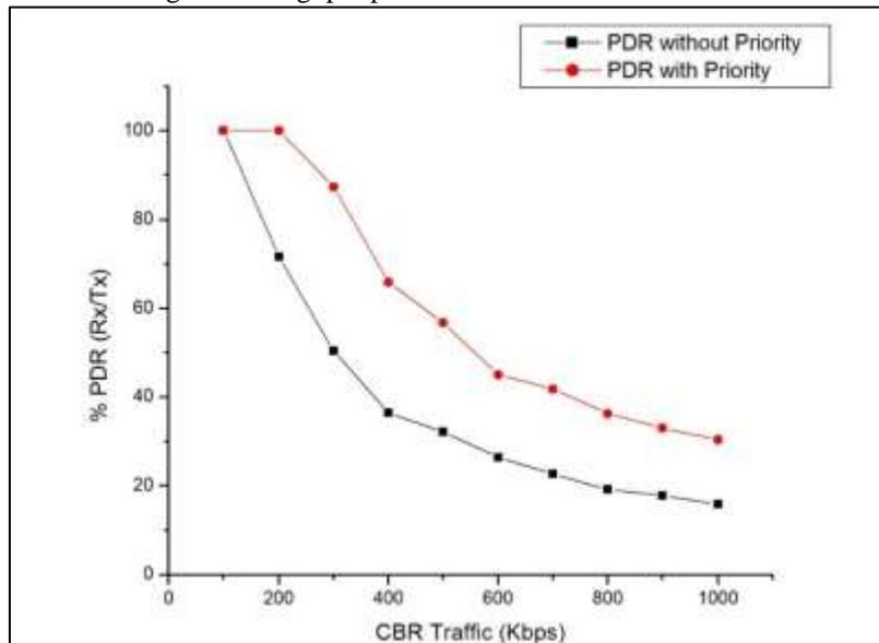
Fig. 3: Packet Delivery Ratio of EDCA over DCF
