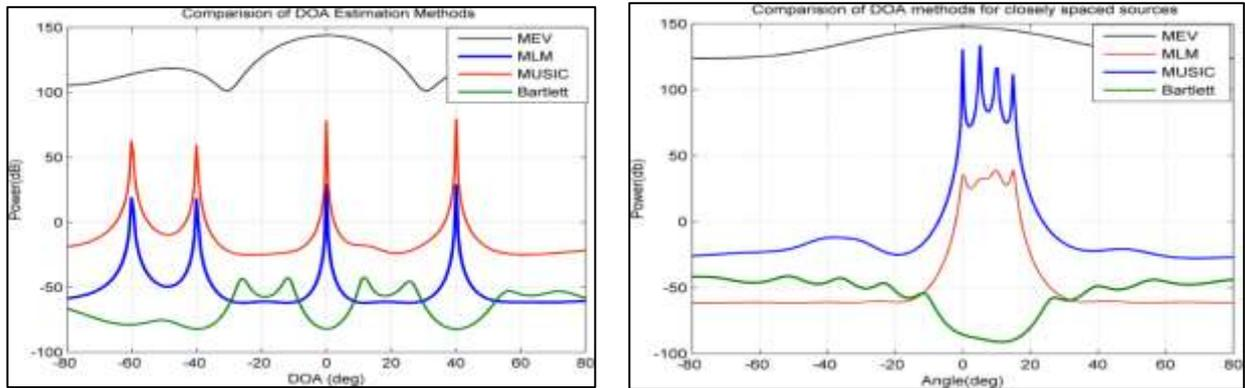
Fig. 8: Comparison of classical and subspace method for DOA estimation.
