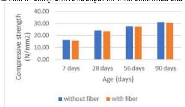
Fig. 2: Comparison of compressive strength for both controlled and SFRC concrete
