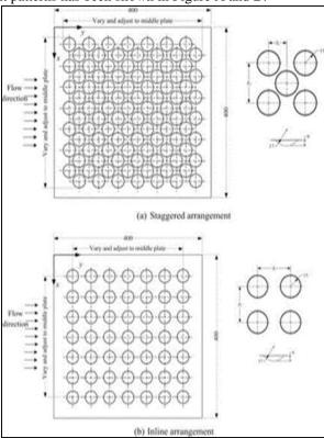
Since the usage of baffles, fins and turbulizers for the conventional enhanced heat transfer approaches results in a significant pressure drop of the stream, the dimples are preferred. In this paper, the dimple arrangements (staggered and inline) with various dimple pitches are compared and studied. The staggered dimple arrangement (Dimple pitches – SL/Dminor = 1.875 and ST/Dminor = 1.875) had been found to provide optimal thermal resistance about 21.7% better than flat plate [1].
