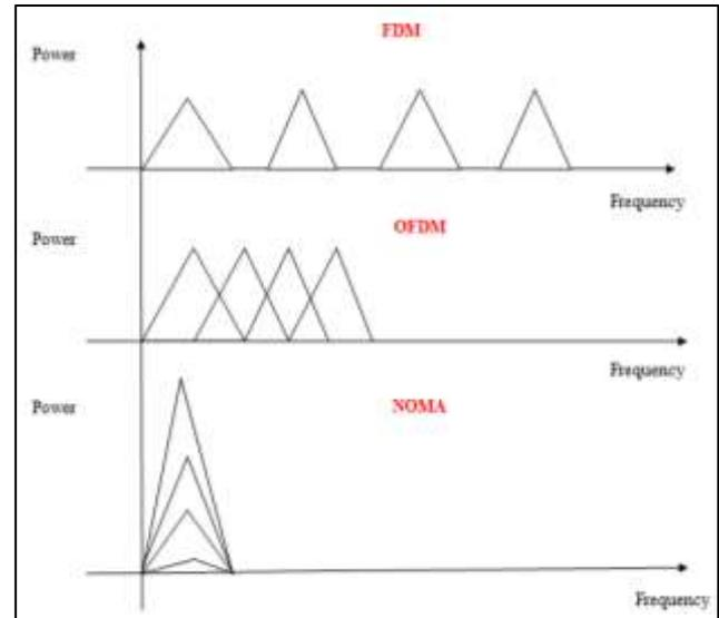
Fig. 1: Spectral of FDM, OFDM and NOMA [3]
