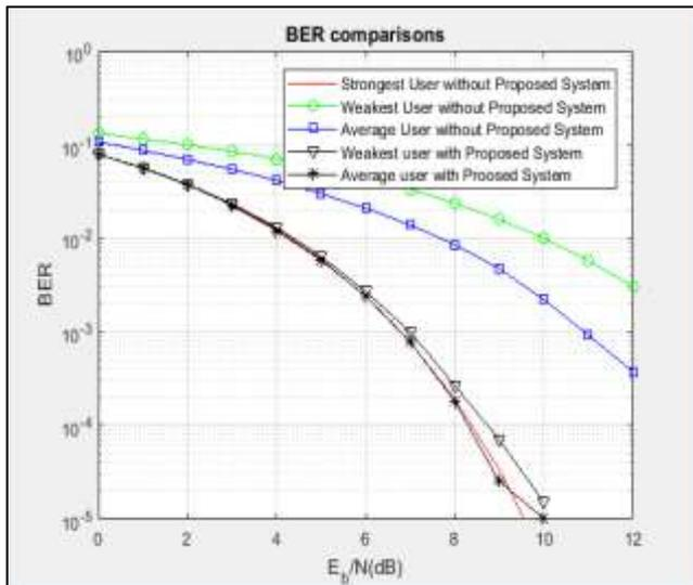
Fig. 5: Obtained BER for the proposed system
