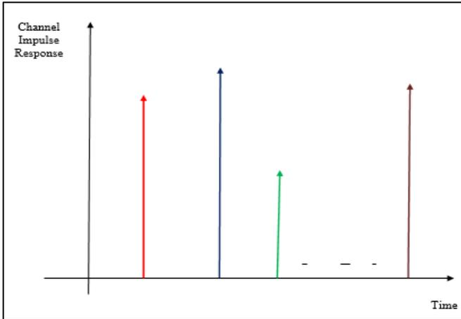
Fig. 2: Temporal Impulse Response of a frequency Selective Channel [4]
