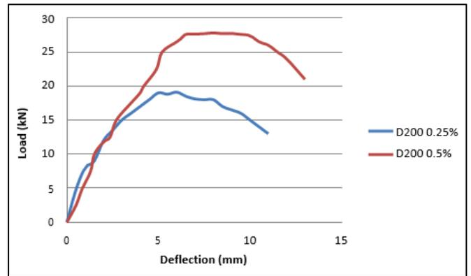
Fig.5.4: Load deflection curves for beams D200 0.25% and 0.5%
