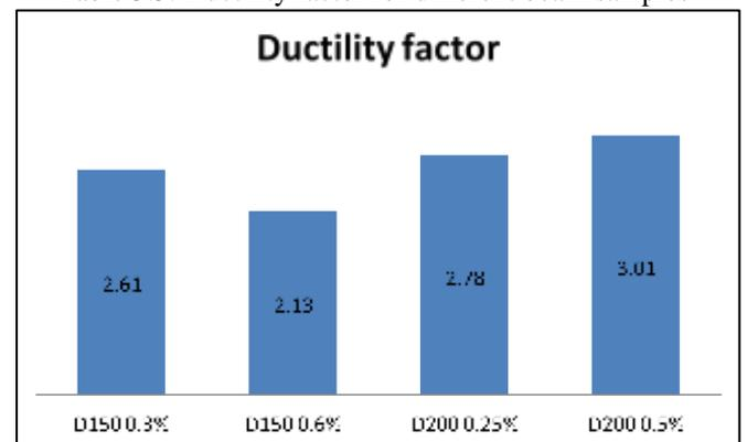
Fig. 5.5: Ductility factors for beam samples
