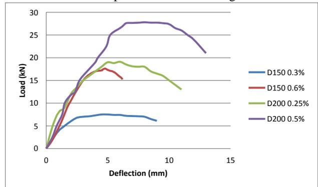
Fig. 5.1: Load vs Deflection curves of RCC beams
