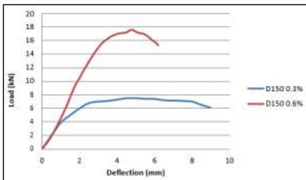
Fig.5.3: Load deflection curves for beams D150 0.3% and D150 0.6%
