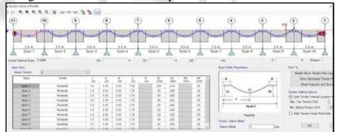
Fig. 4: Longitudinal direction profile of tendon in flat slab
