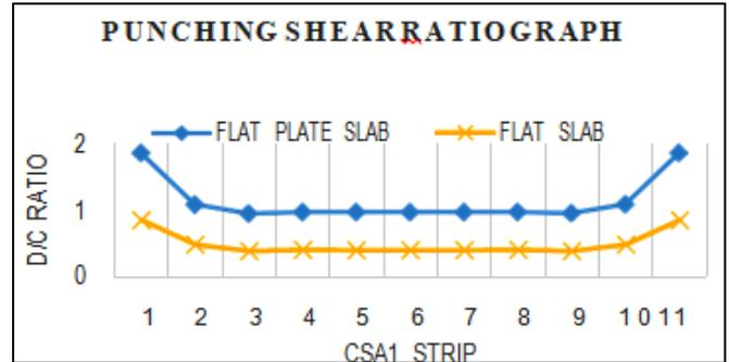
Fig. 10: Punching shear ratio for CSA1 strip columns
