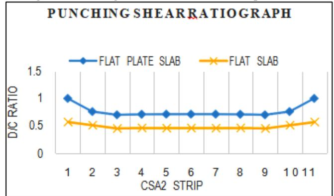
Fig. 11: Punching shear ratio for CSA2 strip columns
