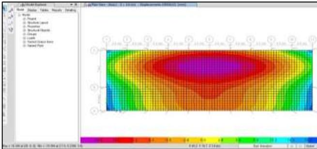
Fig. 8: vertical displacement of flat slab
