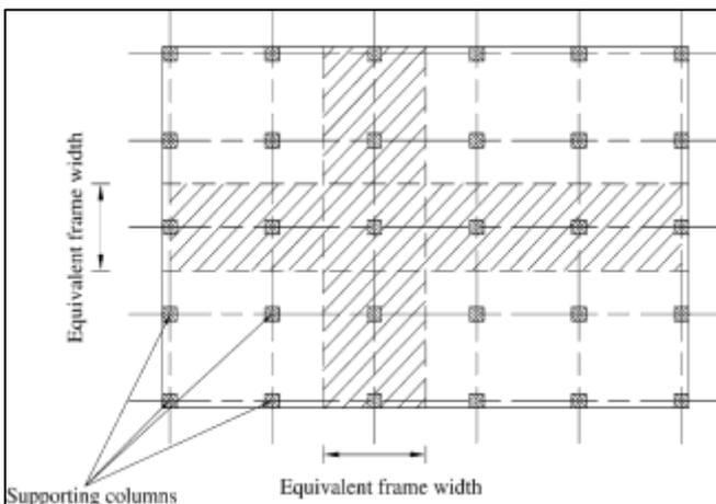
Fig. 1: Plan view of flat plate slab
