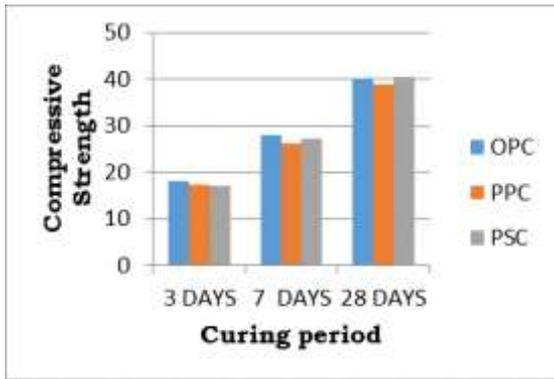
Fig. 1: Comparison for OPC, PPC and PSC in normal water curing
