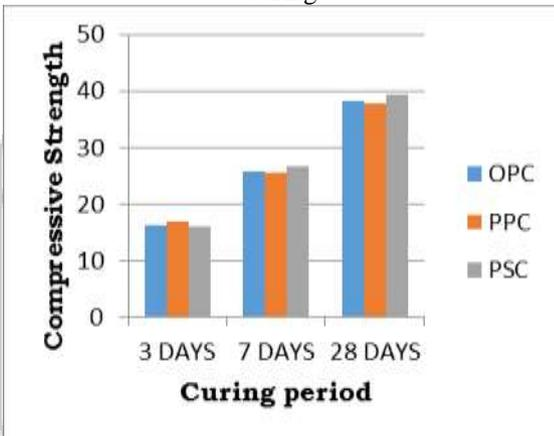
Fig. 2: Comparison for OPC, PPC and PSC in sea water curing
