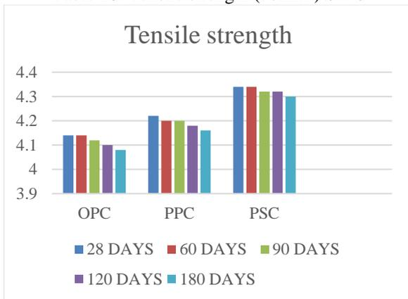
Fig 12 Tensile strength (Sea water curing)
