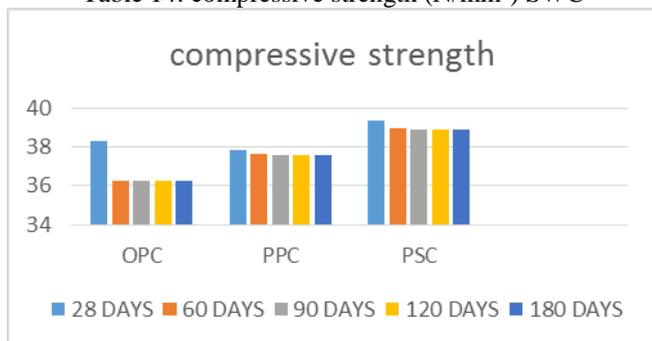
Fig 8: compressive strength (Sea water curing)
