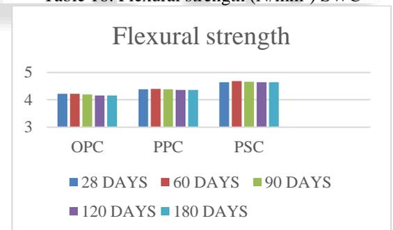
Fig 10: Flexural strength (Sea water curing)
