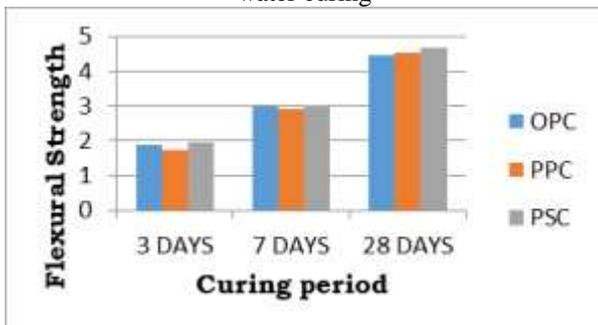
Fig. 3: Comparison for OPC, PPC and PSC in normal water curing
