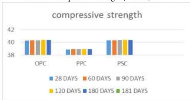
Fig 7: compressive strength (Normal water curing)
