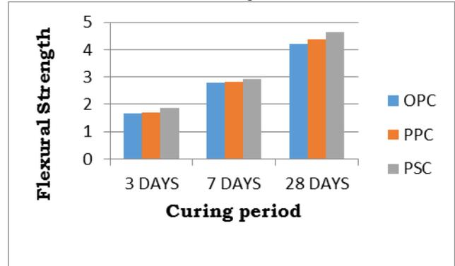
Fig. 4: Comparison for OPC, PPC and PSC in sea water curing
