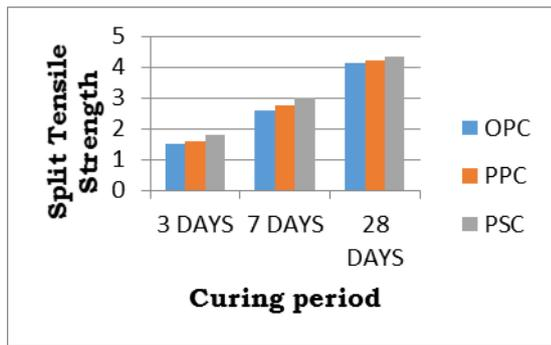
Fig. 6: Comparison for OPC, PPC and PSC in sea water curing
