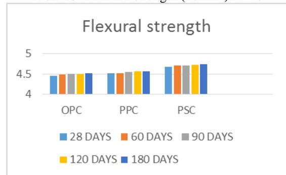
Fig 9: Flexural strength (Normal water curing)
