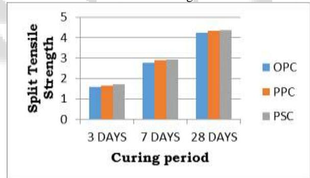
Fig. 5: Comparison for OPC, PPC and PSC in normal water curing
