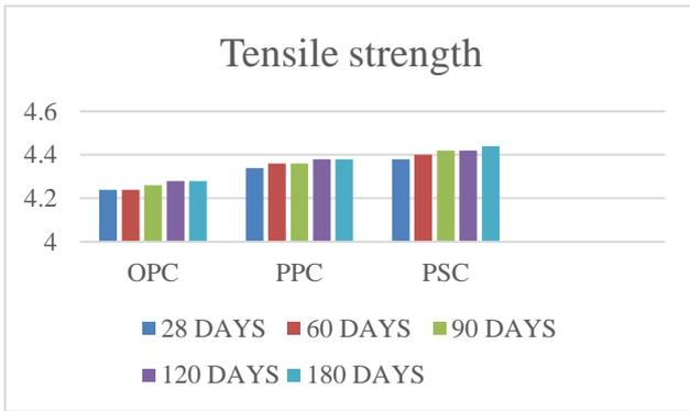
Fig 11: Tensile strength (Normal water curing)
