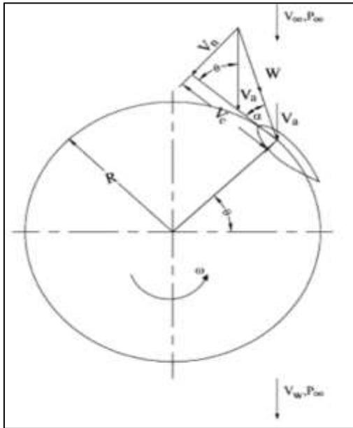
Fig. 1.2: Flow velocities of straight-bladed Darrieus VAWT
