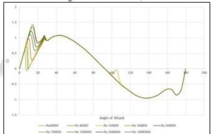
Fig. 1.4: Relation between Blade lift coefficient ( $C_l$ ), Reynold Number ( $Re$ ) & Angle of Attack
