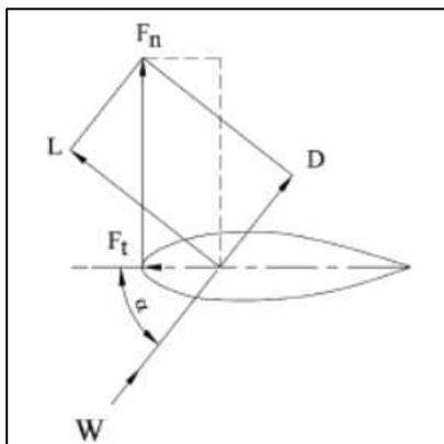
Fig. 1.3: Force diagram of an airfoil
