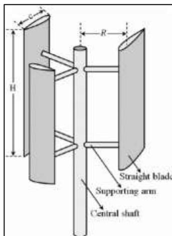
Fig. 1.1: Straight blade Wind Turbine
