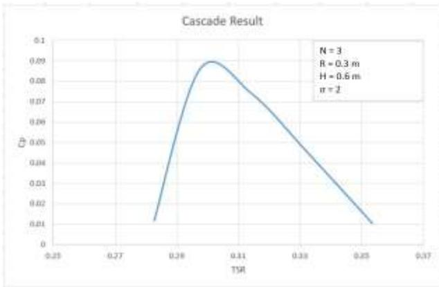
Fig. 1.5: Relation between Coefficient of power ( $C_p$ ) and Tip speed Ratio (TSR)
