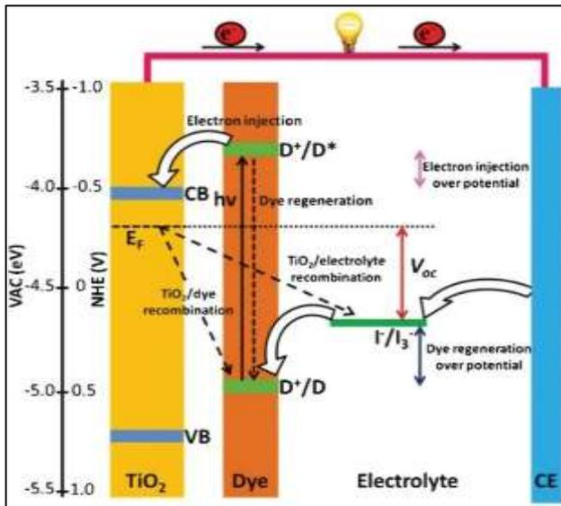
Fig. 4: Energy-level diagram of a DSSC. VAC = vacuum energy level, CB=conduction band, VB=valenceband
