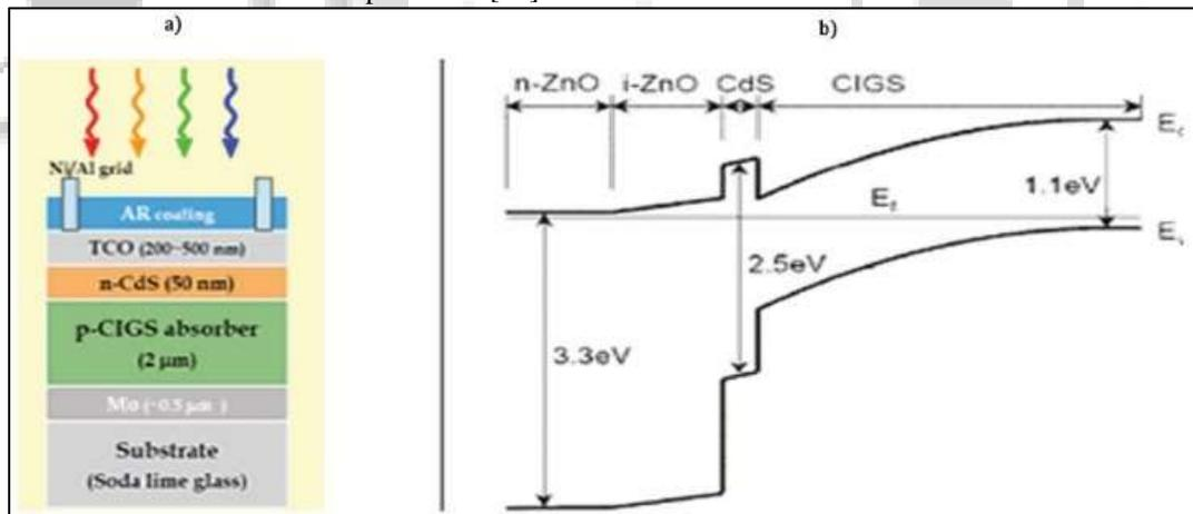
Fig. 3: (a) Basic structure of a CIGS solar cell (b) CIGS solar cell band diagram.
