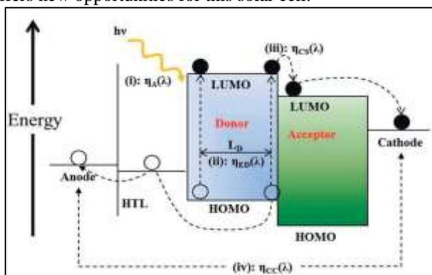
Fig. 5: Mechanism of an organic solar cell
