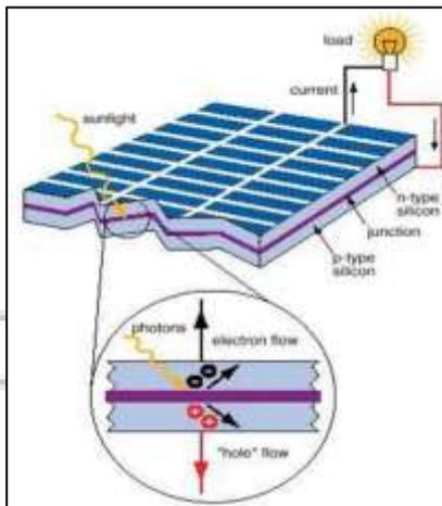
Fig. 2: Structure of silicon solar cell adapted from [12].
