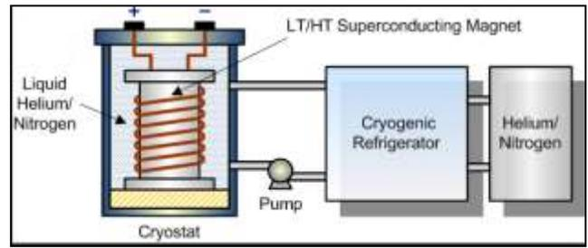
Fig. 4.1: Cryogenic Unit
