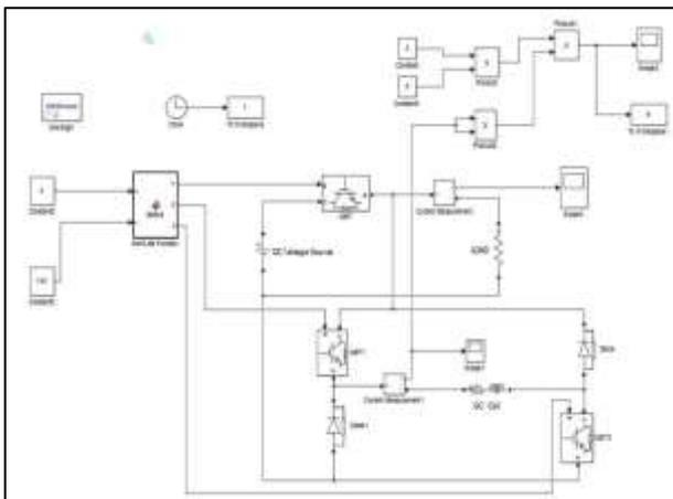
Fig. 5.1: Matlab simulation diagram proposed DC SMES System for high voltage Operation
