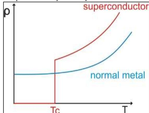
Fig. 2.1: Characteristics Diagram of Super conductivity
