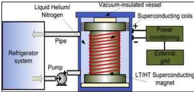
Fig. 3.1: Schematic diagram of SMES system
