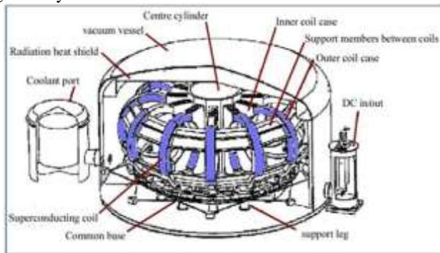
Fig. 3.2: Main Parts of SMES System
