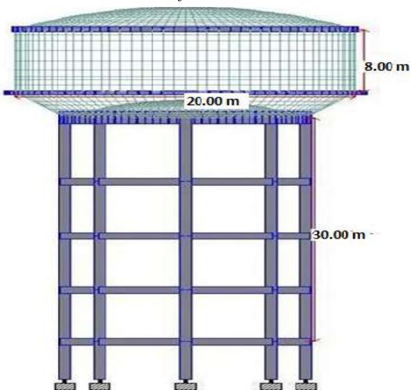
Fig. 4.5: FEM Model of Elevated Water tank
