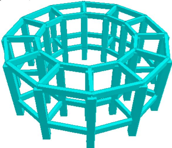
Fig. 4.6: Concentric columns type of staging
