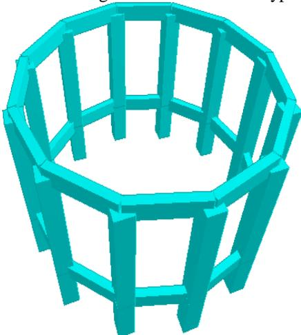
Fig. 4.8: Radial Bracing type of staging
