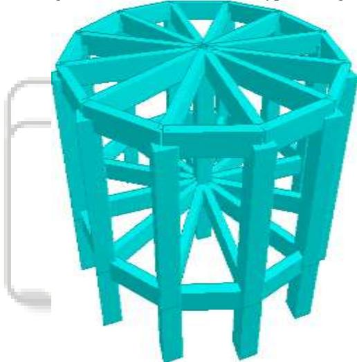
Fig. 4.7: Radial Bracing with central column type of staging
