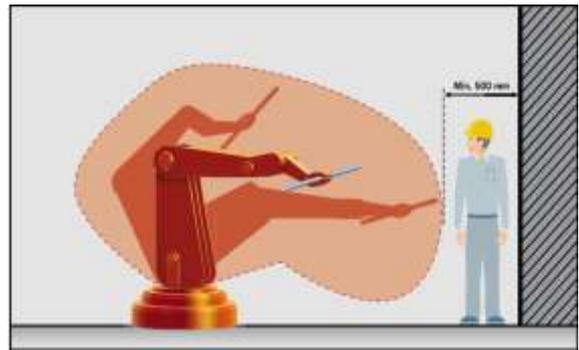
Fig. 4: minimum gaps between the Robot and Guard [38]
