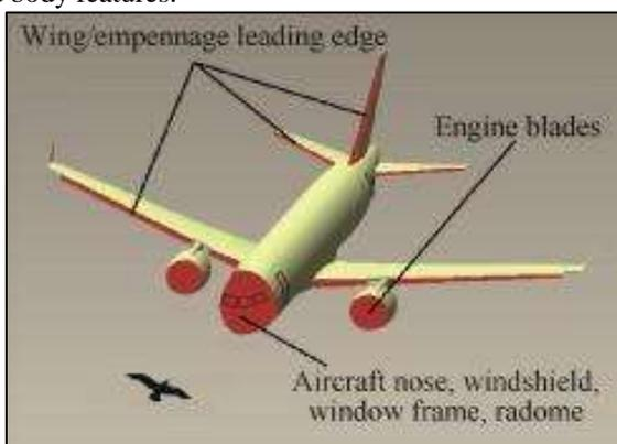
Fig. 1: Design of aircraft structures against threat of bird strikes
