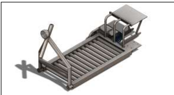
Fig. 4: Main Frame / Chassis
