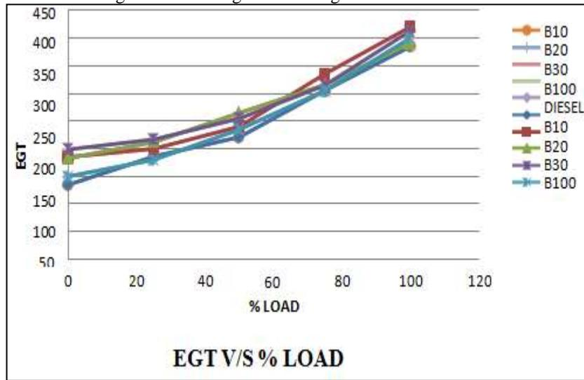
Fig. 6: Exhaust gas temperature v/s % load
