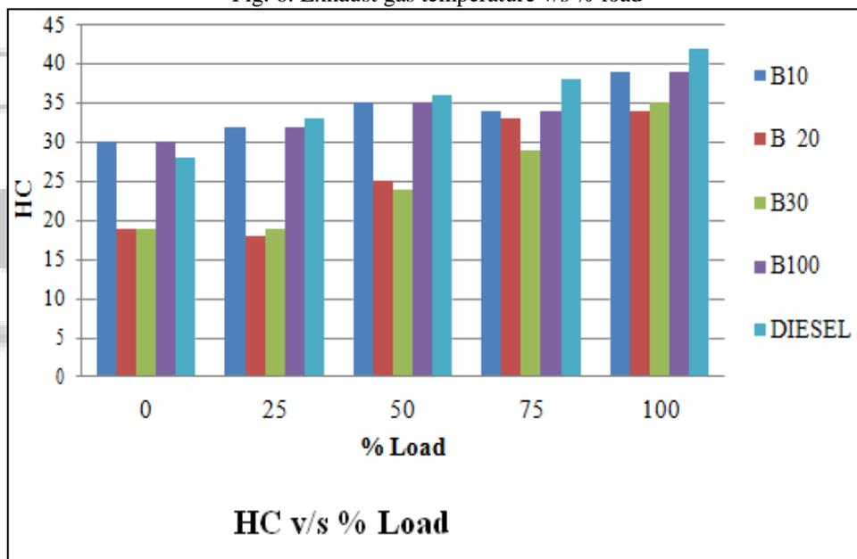
Fig. 7: HC Emission in ppm for spent coffee powder biodiesel
