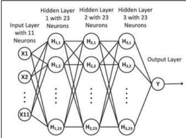
Fig. 1: Neural network proposed architecture
