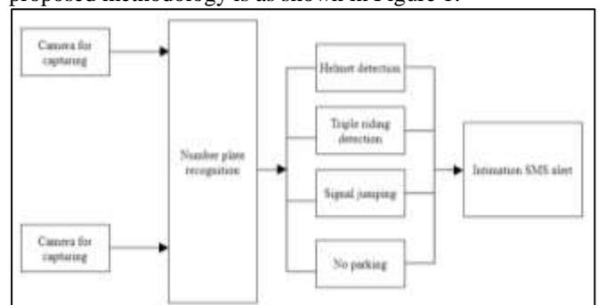
Fig. 1: Proposed block diagram for violation detection.
