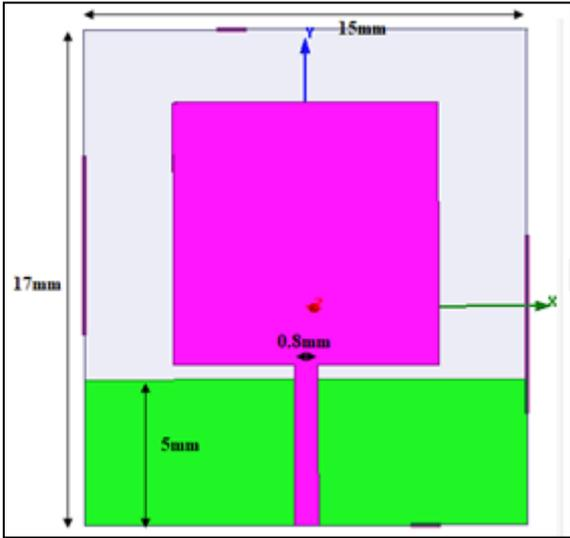
Fig. 1: Microstrip monopole antenna
