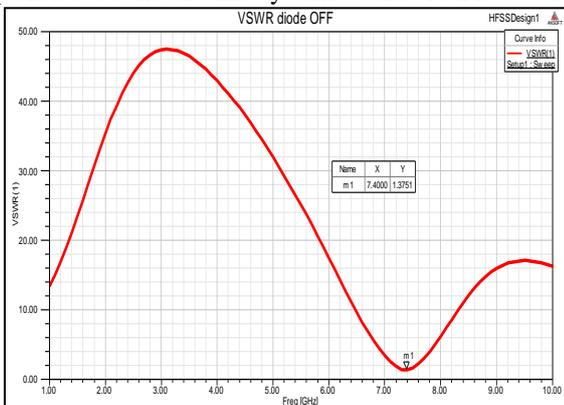
Fig. 3: VSWR when diode is OFF
