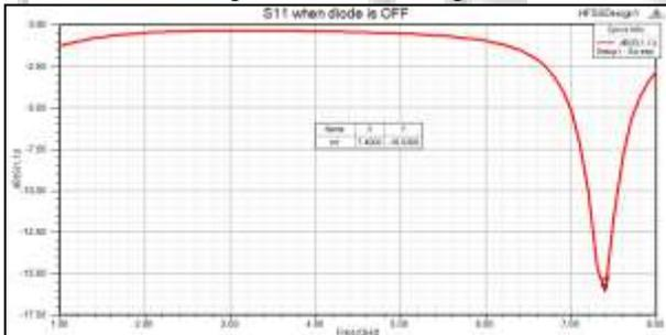
Fig. 2: Return loss plot when diode is OFF
