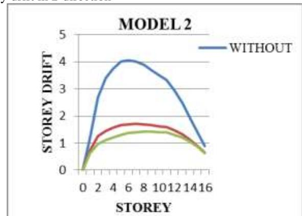
Chart 10: Comparison of storey drift in z direction
