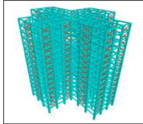
Fig. 4: Plus Shape model 1 with arrangement of Bracing system
