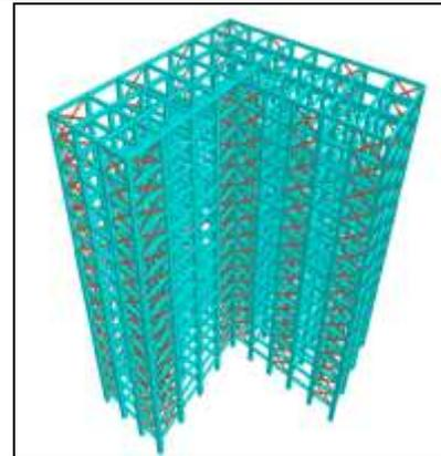
Fig. 2: L Shape model 1 with arrangement of Bracing system
