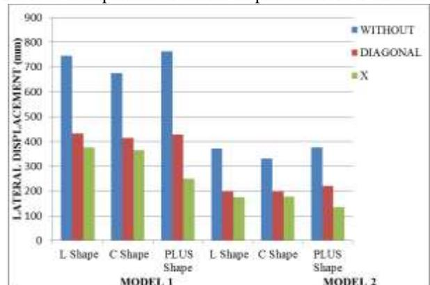
Chart 1: Comparison of lateral displacement in x-direction
