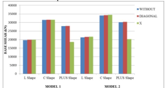
Chart 16: Comparison of base shear in z-direction
