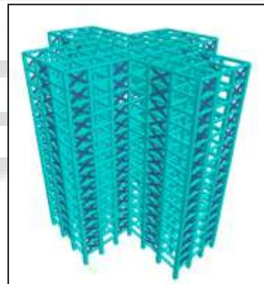
Fig. 7: Plus Shape model 2 with arrangement of Bracing system
