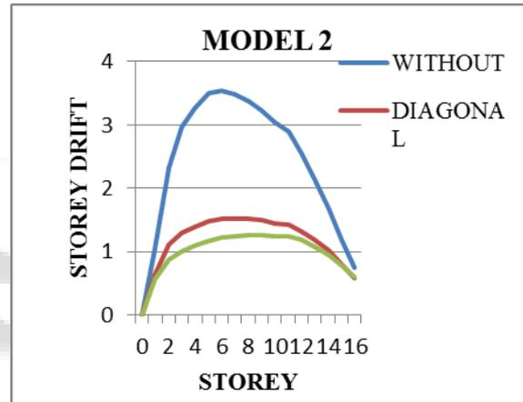
Chart 6: Comparison of storey drift in z-direction
