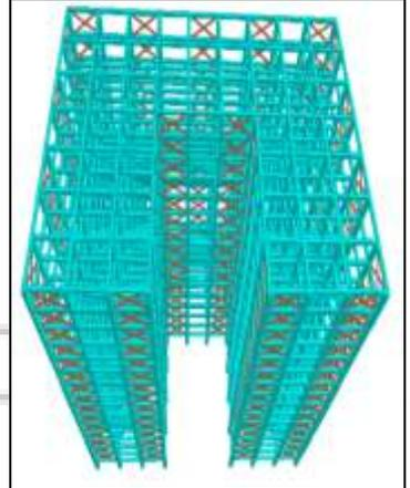
Fig. 3: C Shape model 1 with arrangement of Bracing system
