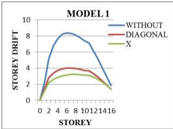
Chart 13: Comparison of storey drift in z-direction
