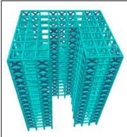
Fig. 6: C Shape model 2 with arrangement of Bracing system
