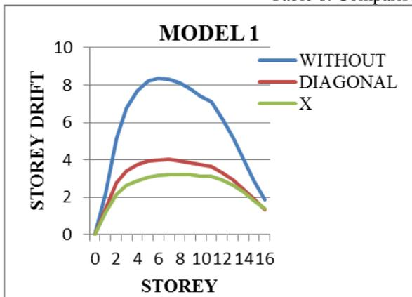
Chart 9: Comparison of storey drift in z direction
