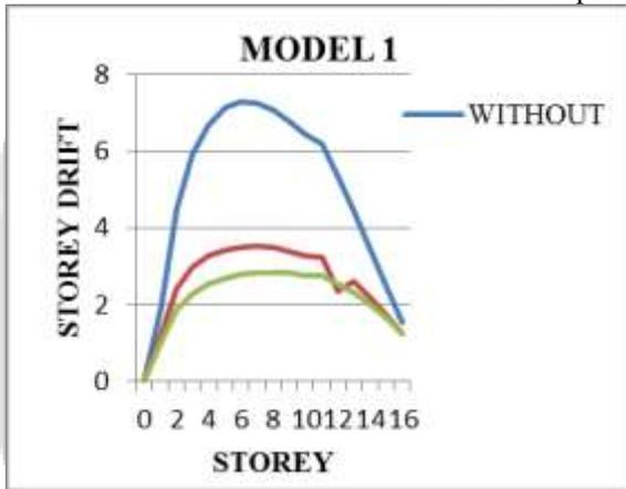
Chart 5: Comparison of storey drift in z-direction
