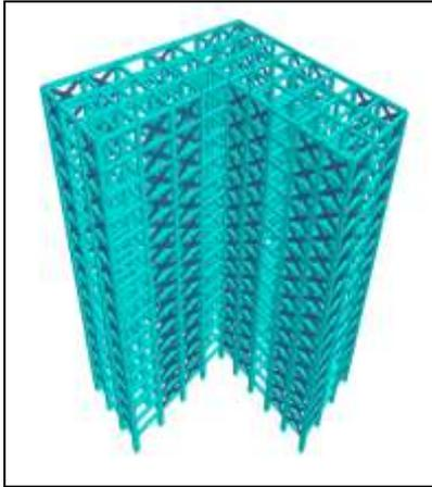
Fig. 5: L Shape model 2 with arrangement of Bracing system
