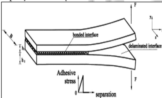
When size of delamination is small, minor changes in natural frequency are resulted. It was observed that effect of multiple delaminations is more significant than that for single delamination. Declining frequency trend was concluded for constrained mode shape model. When a delamination occurs at the mid plane, minimum value of non-dimensional fundamental frequencies are resulted.
