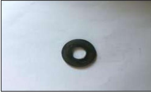
Spring washers, also called disc springs or conical washers use spring loads to create axial flexibility. This counteracts settlements and maintains an initial level of preload. The washers are installed between the bolt head/nut and the mating surface.
