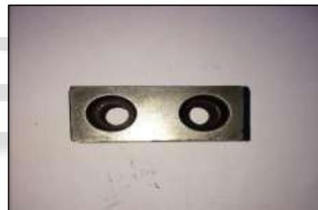
Rest pads are used in fixture and jig construction as support and locating elements. They can be used as feet, supports, side locators, and wear points. They are also known as rest buttons and thrust bolts
