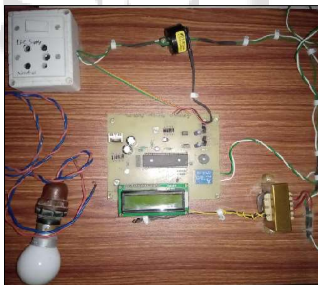
Fig. 3 a): View of Intelligent Electrical Protector
