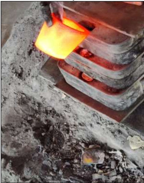
Fig. 2: Graphite crucible in sand casting process
