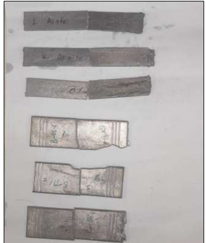
Fig. 3: Al+Fe and Al+Fe+Zr samples after testing
