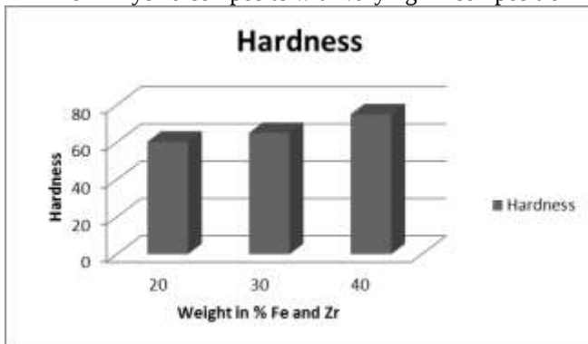
Fig. 8: Behaviour of Al+Fe+Zr hybrid composite on hardness with varying Iron and Zirconium composition
