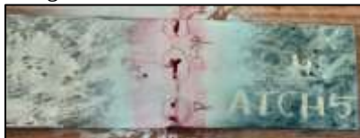
Fig. 3.2: Defects on root of weld
