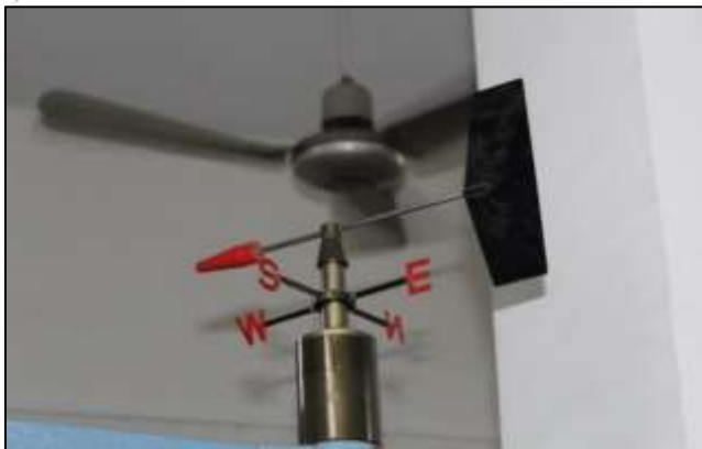
Fig. 2: Potentiometric Wind Vane
