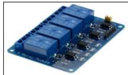
Fig. 4: Relay Module of 4 channel 5 volts
