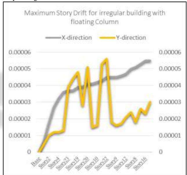
Fig. 6: Maximum Story Drift for irregular building with floating Column
