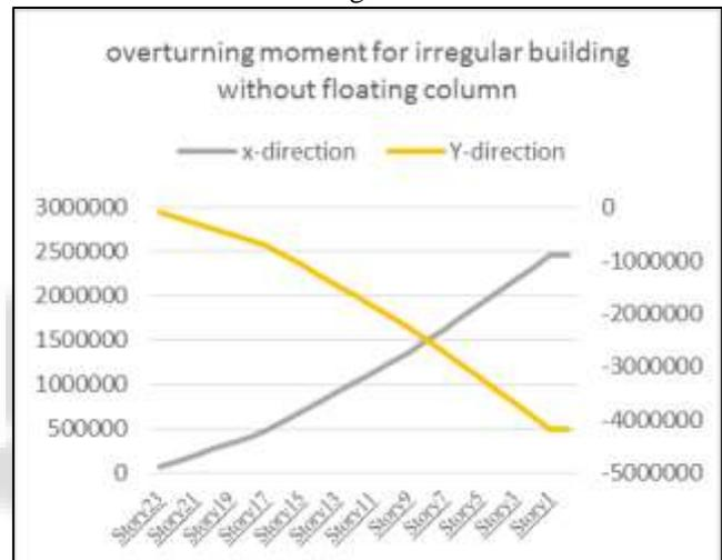
Fig. 11: overturning moment for irregular building without floating column
