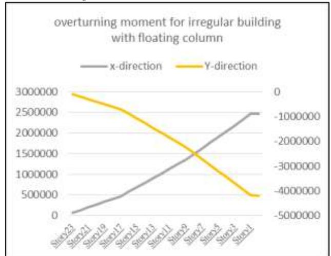
Fig 10: overturning moment for irregular building with floating column
