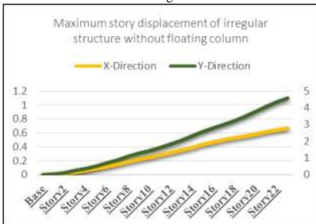
Fig. 5: Maximum story displacement of irregular structure without floating column
