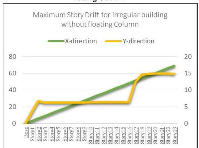
Fig. 7: Maximum Story Drift for irregular building without floating Column
