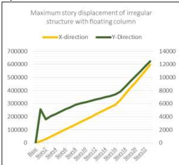
Fig. 4: Maximum story displacement of irregular structure with floating column
