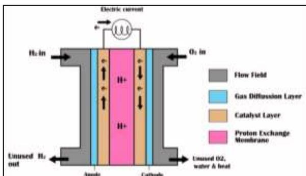
Fig.1: Structure of PEMFC
