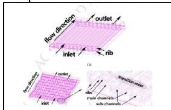
Fig. 7: 3D cathode flow field with main and sub-channels [6]
