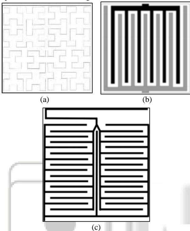
Fig. 16: (a) Fractal geometry, (b) Lung-shaped flow field, (c) Murray interdigitated flow field [15]
