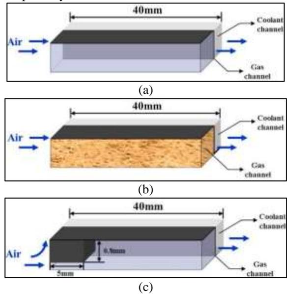
Fig. 17: (a) Cathode flow field- parallel, (b) Cathode flow field with metal foam, (c) Cathode flow field reduced inlet [17]
