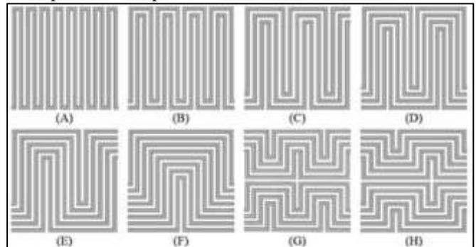
Fig.11: (a) Single channel, (b) 2 channels, (c) 3 channels, (d) 4 channels, (e) 5 channels, (f) 8 channels (g) Modified serpentine flow field with 4 channels, (h) Modified serpentine flow field with 5 channels [10]
