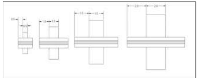
Fig. 5: Front view of PEMFC with four different Landing to Channel width [4]
