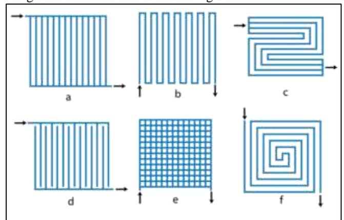
Fig. 2(a) Parallel flow field, (b) Serpentine flow field, (c) Multi-pass channel of serpentine flow field, (d) Interdigitated flow field, (e) Pin-type flow field, (f) Spiral flow field
