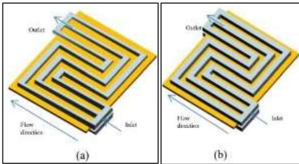
Fig. 12: (a) Modified serpentine flow field, (b) Serpentine flow field [11]
