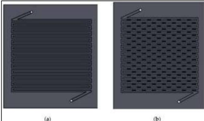
Fig. 19: (a) Serpentine flow field, (b) Modified Serpentine with Staggered provisions of 4 mm porous sponge inserts Flow Field [19]
