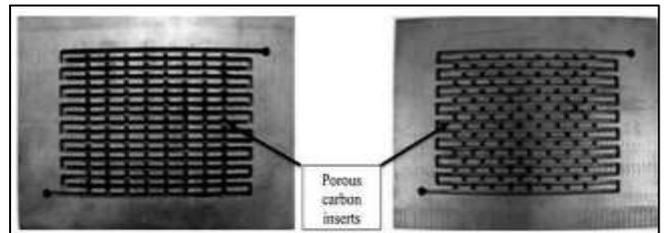
Fig. 10: Adoption of porous carbon inserts on the PEMFC with active area of 70cm<sup>2</sup> in (a) Uniform pin type flow field, (b) Zigzag pin type flow field. [9]
