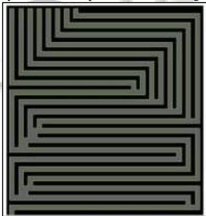
Fig. 20: Cascade type flow field [20]
