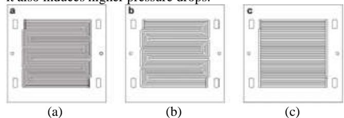
Fig. 18: (a) 5 step serpentine pattern, (b) 4 step serpentine patterns, (c) Parallel channel pattern [18]
