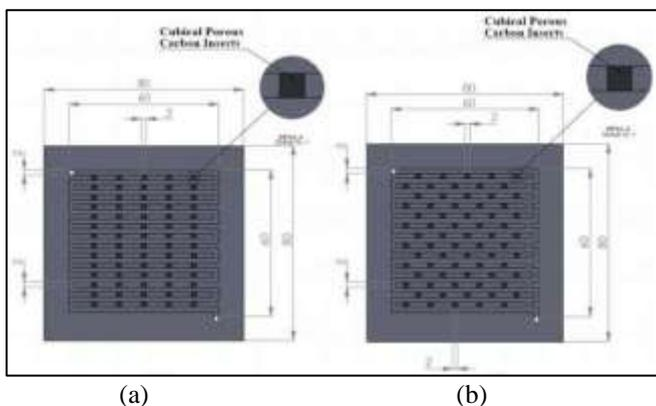
Fig. 9: Flow field designs of 36 cm<sup>2</sup> active area (a) Uniform patterned pin type with porous inserts, (b) Stagger patterned pin type with porous inserts. [8]
