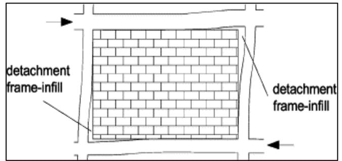
Fig. 1: Behaviour of walls under lateral loading
