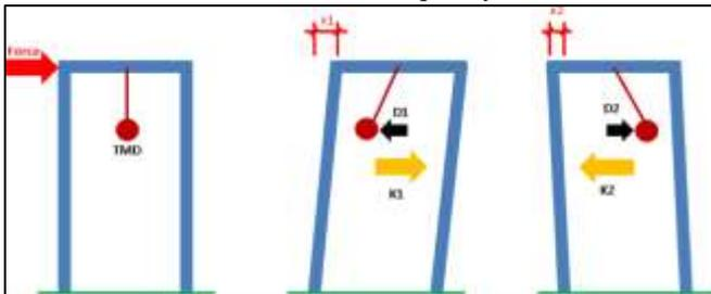
Fig. 3: Movement of TMD under lateral loading
