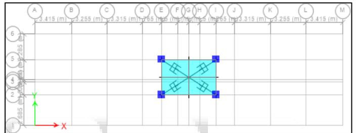
Fig. 8: Plan with TMD at top storey with TMD and Pistons
