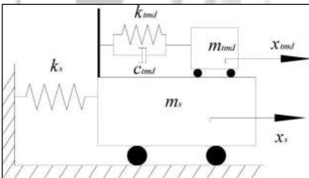
Fig. 4: Schematic diagram of Primary structure and TMD using D'Alembert's principle of equilibrium equation
