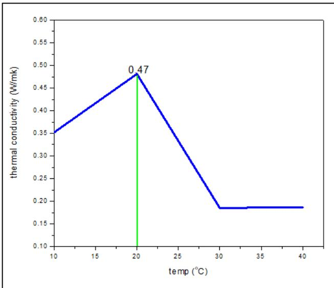
Fig. 10: Thermal conductivity graph for PEG-600
