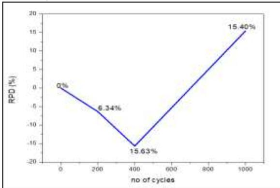
Fig. 5: Variation of melting point after thermal cycling.
