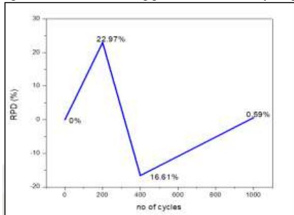
Fig. 6: Variation of the latent heat after thermal cycling.
