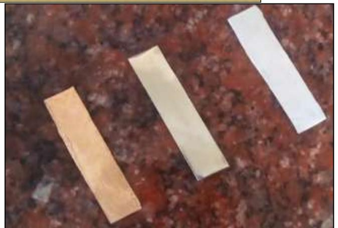
Fig. 11: Cu, Al, and stainless steel 316 specimen before testing.
