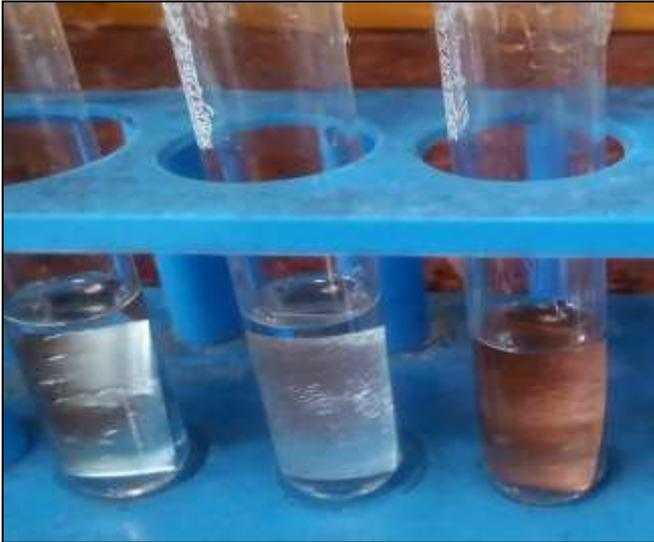
Fig. 1: S.S, Al, Cu samples dipped in PEF-600
