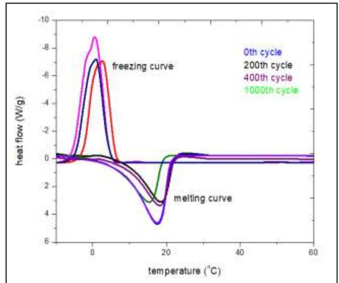
Fig. 7: DSC curves of the PCM 0, 200, 400, 1000 thermal cycles.
