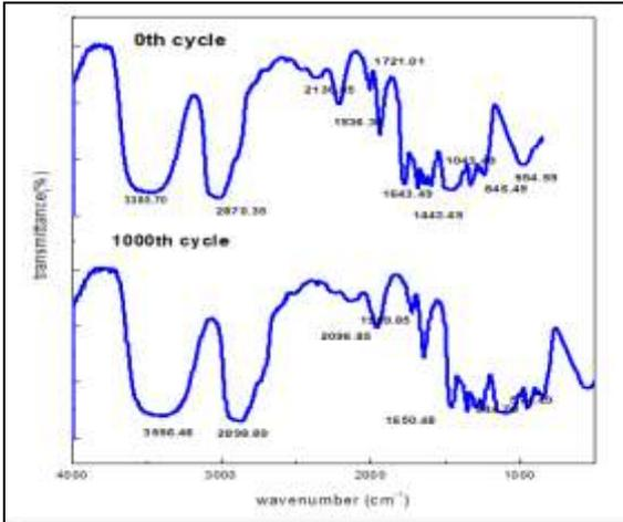
Fig. 8: FTIR spectra of PEG-600 after 0 and 1000 cycle.
