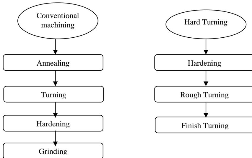
Fig. 2: Comparison between Conventional machine and hard turning [10]
