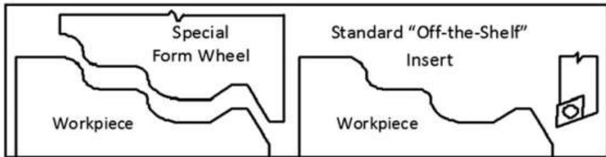
Fig. 1: Grinding versus hard turning [5]
