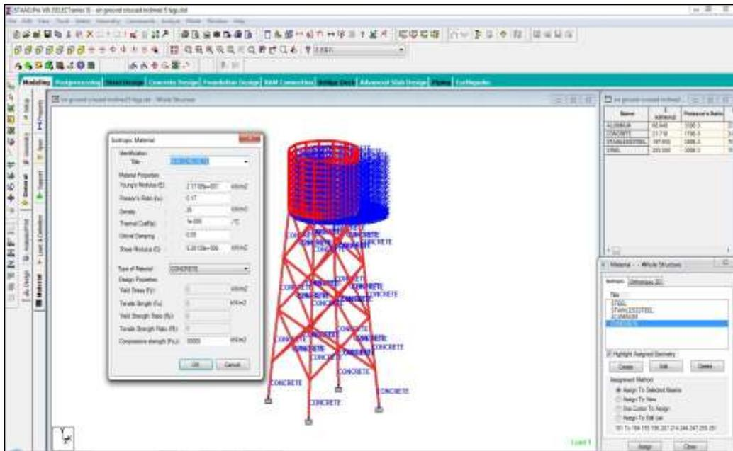
Fig. 2: Assigning Material Properties
