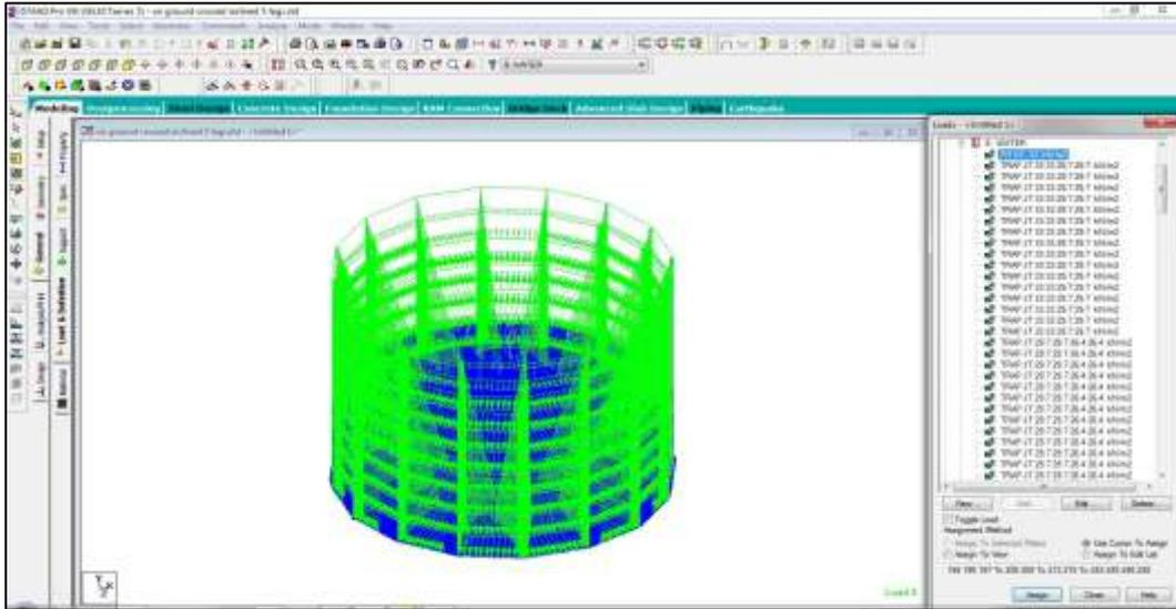
Fig. 5: Assigning Hydrostatic Load
