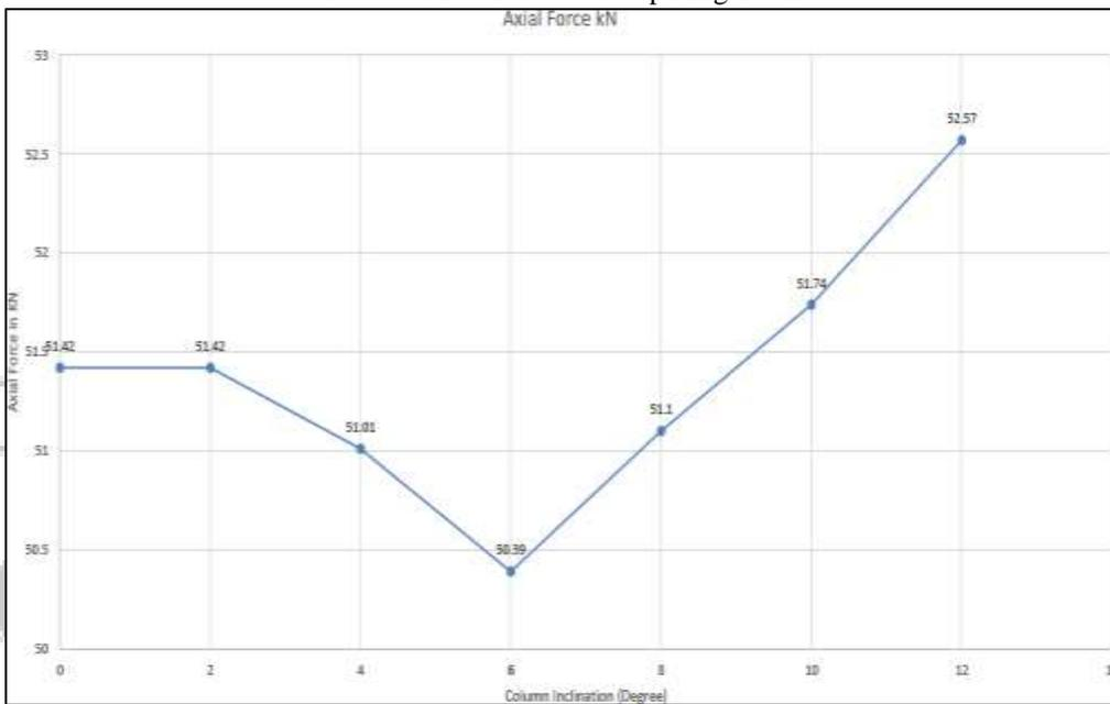
Fig. 8: Axial Force at Top Beam
