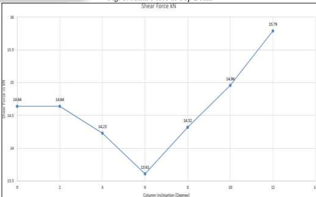
Fig. 9: Shear Force at Top Beam
