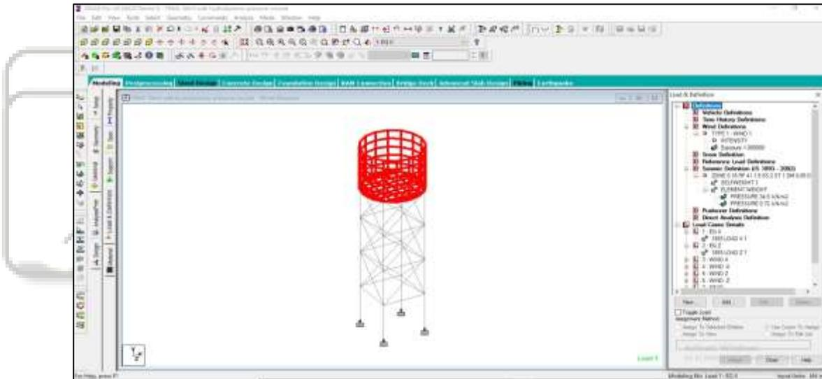
Fig. 6: Assigning Lateral Loads namely wind load and seismic load
