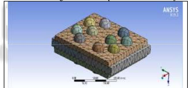
Fig. 5: Meshing of the joint assembly
