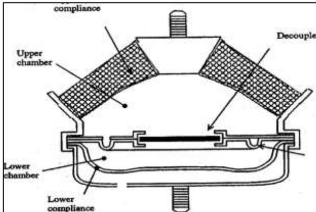
Fig. 5: Sketch view of hydraulic engine mount
