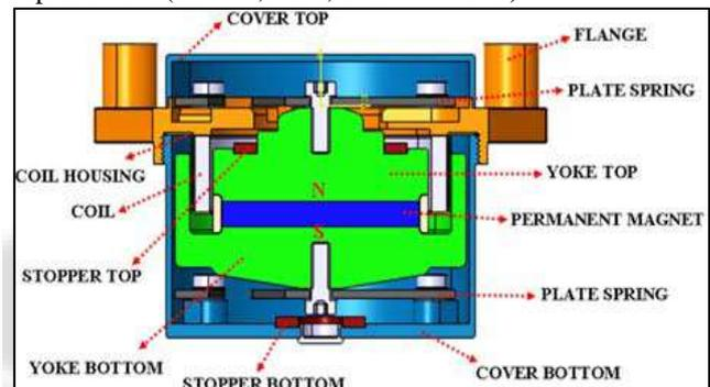
Fig. 5: Voice coil actuated engine mount
