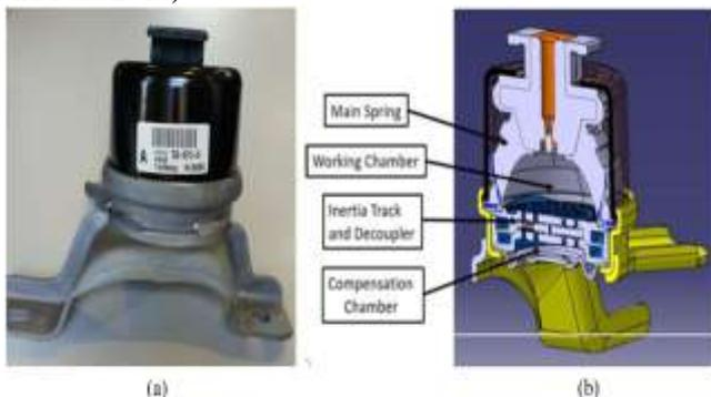
Fig. 6: The hydraulic engine mounting components are shown
