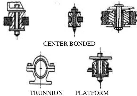
Fig. 2: Typical elastomeric mounts [3]
