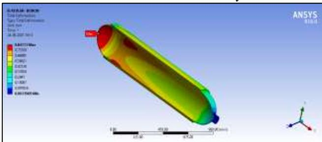
Fig. 1: Axial Deformation of composite gas cylinder under pressure 20 MPa Kevlar & Boron.
