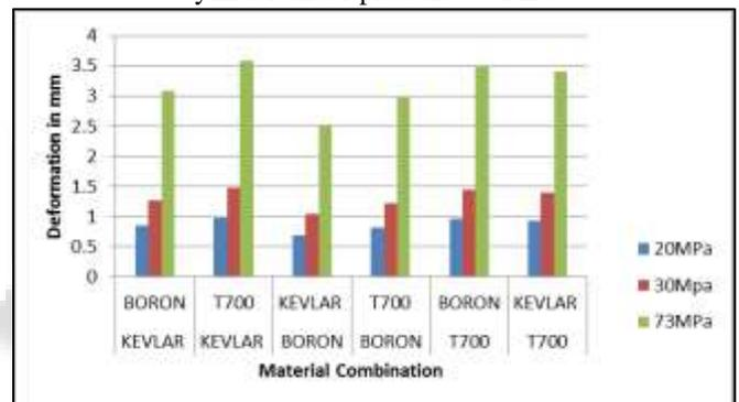
Fig. 4: Axial Deformation of all composite gas cylinder under all three pressure 20MPa, 30 MPa and 73 MPa
