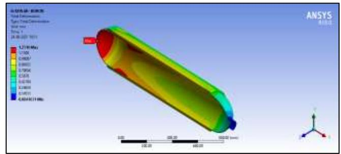
Fig. 2: Axial Deformation of composite gas cylinder under pressure 30 MPa
