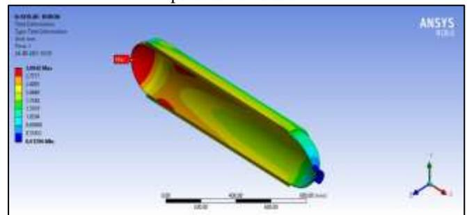
Fig. 3: Equivalent (von-mises) Stress of composite gas cylinder under pressure 73 MPa
