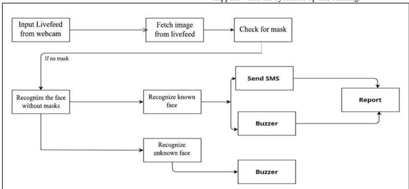
Fig. 1: Block Diagram of Face Mask Detection
