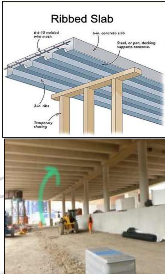
Fig. 2: Typical examples of ribbed slab
