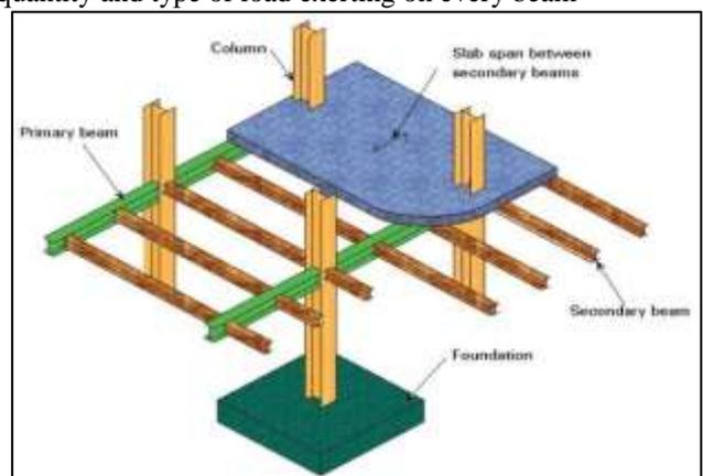
Fig. 4: Structure having secondary beam
