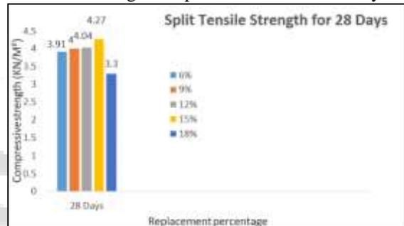
Tensile Strength Graph of Concrete for 28 days
