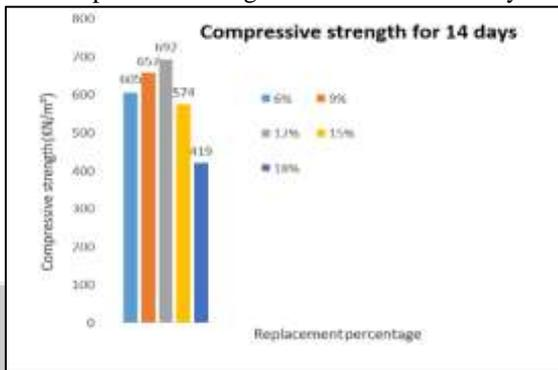
Compressive Strength of Concrete for 14 Days
