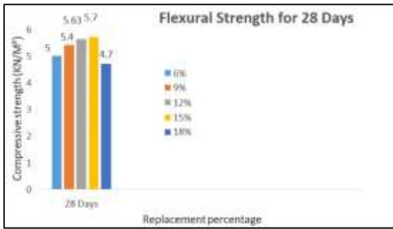
Flexural Strength of Concrete for 28 Days
