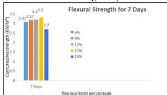
Flexural Strength of Concrete for 7 Days
