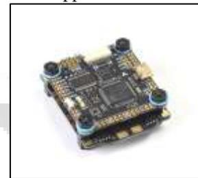
Fig. 2: MPU6000 Flight Controller
