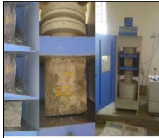
Compressive Strength Test
