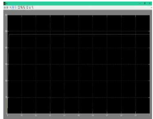
Fig. 6(f): Output voltage of PV module after MPPT
