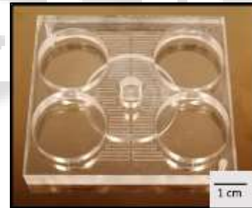
Fig. 2: Final Device with OW. The assembled device is repositioned on the micro-cutter and window is machined with reduced z-pitch for lesser roughness on the rear side
