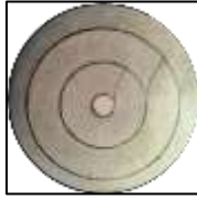
Fig. 3: Detail of the OW under optical microscope. It is visible for the concentric structures created because of milling. Hence, reduction of roughness is obligatory for better visualization
