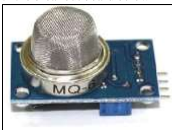
Fig. 7: MQ6Sensor LPG Gas Sensor (MQ6) Features:
