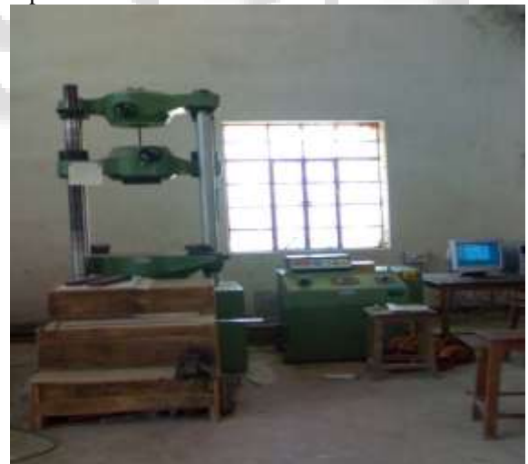
Fig. 6: UTM testing setup
